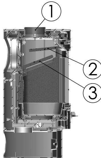
**Make sure that the baffles are correctly assembled before lighting the stove
